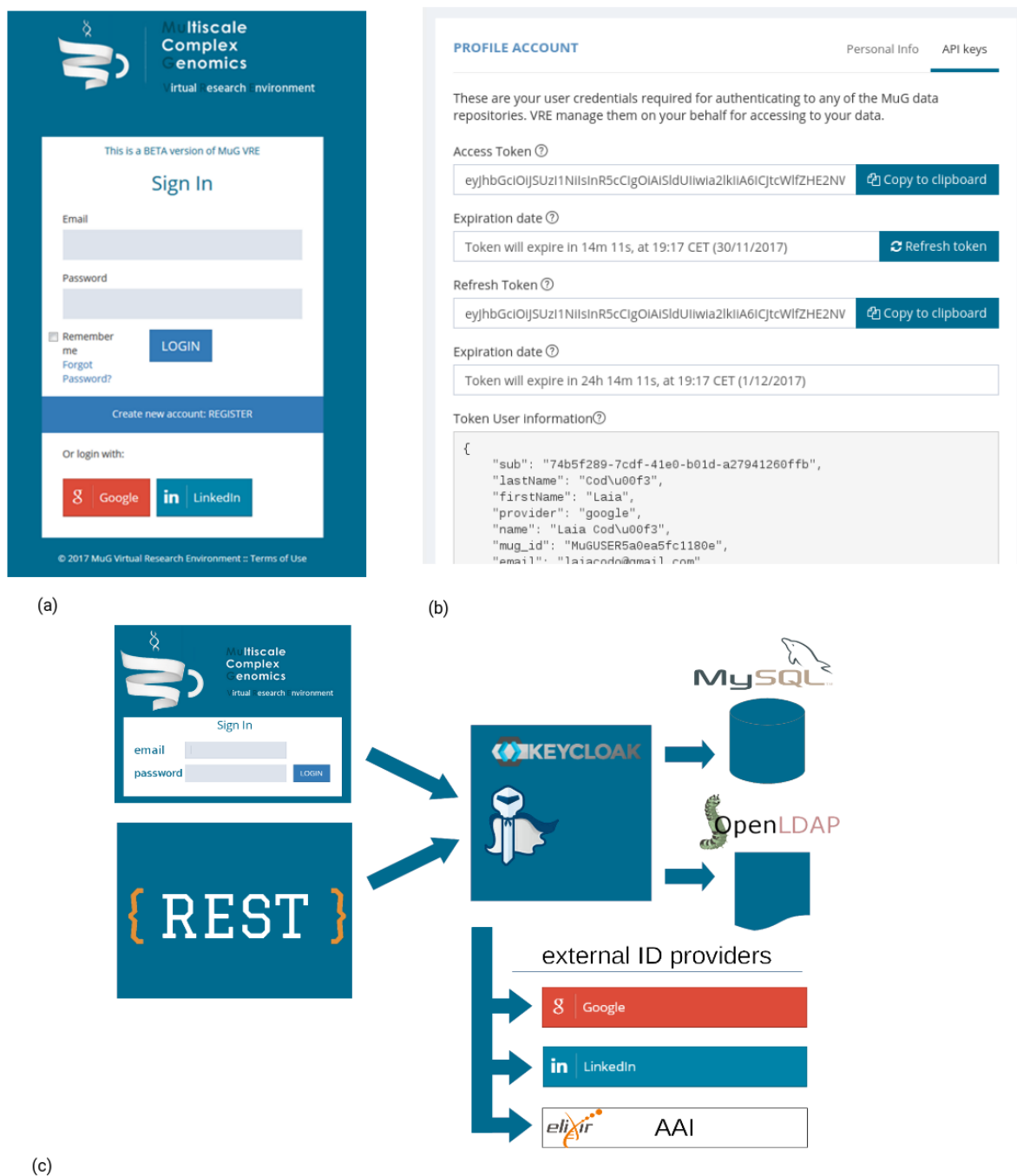
Figure 7. (a) VRE Login page. (b) User profile details including authorization tokens. (c) Schema of the MuG centralized authorization service based on Keycloak
